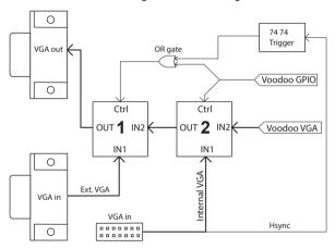
Multiplexer IC chip provides switching VGA signal from IN1 to OUT, when Ctrl pin state is low and IN2 to OUT, when Ctrl state is high.
